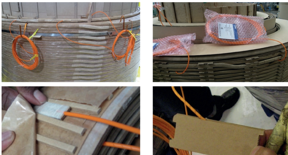
Figure 4 – Typical fiber optic probe installation in transformer winding spacers. Proper installation ensures sensor durability and measurement accuracy.
