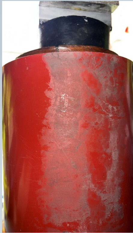
Figures 3, 4 & 5 - Further evidence of electrical tracking along composite insulator tube (Left) and internal view of inner insulation liner/bonding layer showing damage as a result of electrical discharge due to loss of equipotential bond (Right Upper & Lower).
