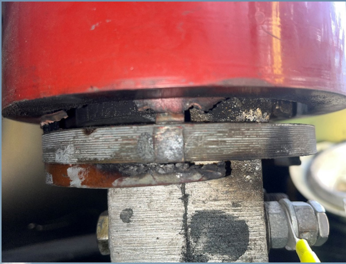
Figures 1 & 2 - IPB Mounted Current Transformer (CT) showing evidence of damage to equipotential bonding ring, inner insulation sleeve and tracking marks (treeing) in composite insulator.
