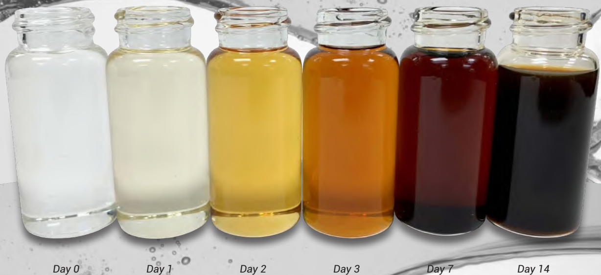
Mineral oil sample performance under test: ageing and oxidation
