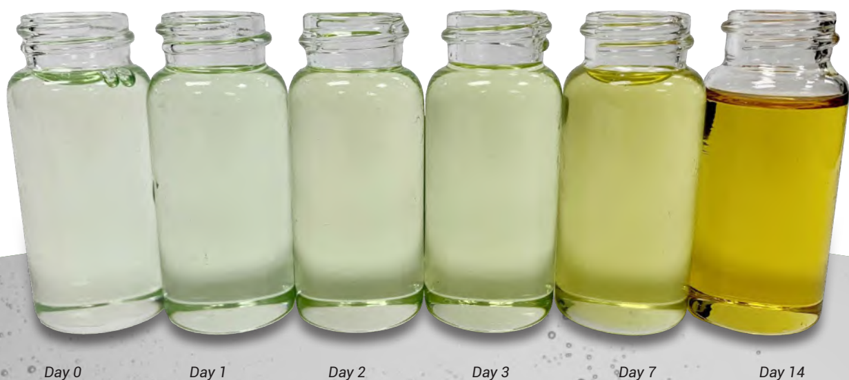
FR3 fluid sample performance under test: ageing and oxidation
