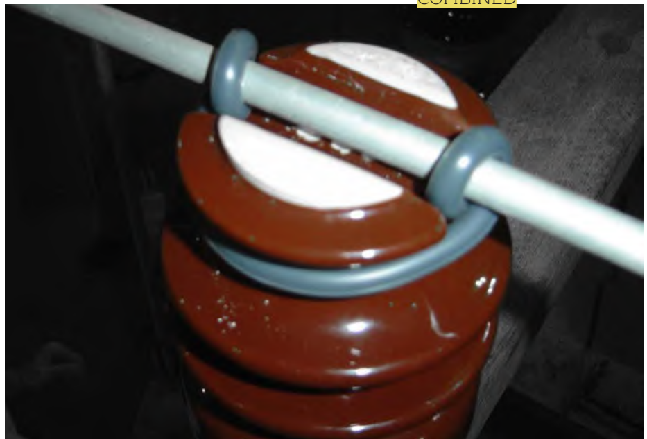
Figure 2. Tracking has begun to erode the enamel coating on this insulator. Moisture can impregnate and either super heat (arcing) or freeze. The insulative properties are failing and partial discharge will only worsen from here.
