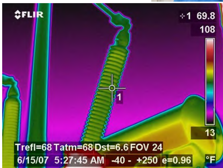
Figure 3. Infrared did not discover any electrical anomalies; however, additional ultrasound scans revealed the onset of early stages of corona discharge.
