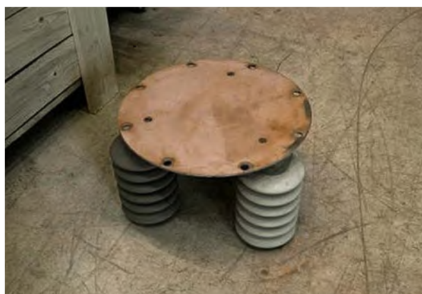
Figure 4. Electrode and test setup used for testing gaps up to 150 mm.
