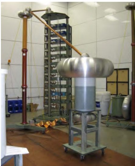
Figure 2. Test setup and electrodes for testing the interfacial creep breakdowns.
