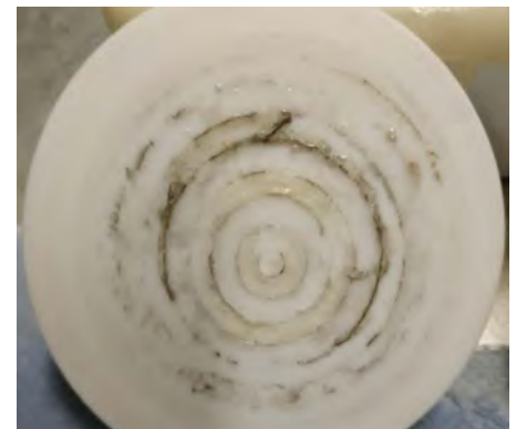
Figure 8. The charts (left) present the different profile for the partial discharges. The photos (right) show the solidified materials formed after the 200 h of ageing under PDs.
