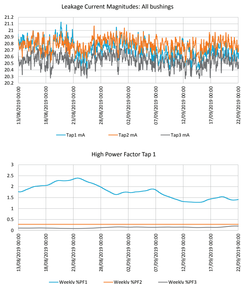
Figure 5. Leakage Current and Relative Power factor for failing bushing
