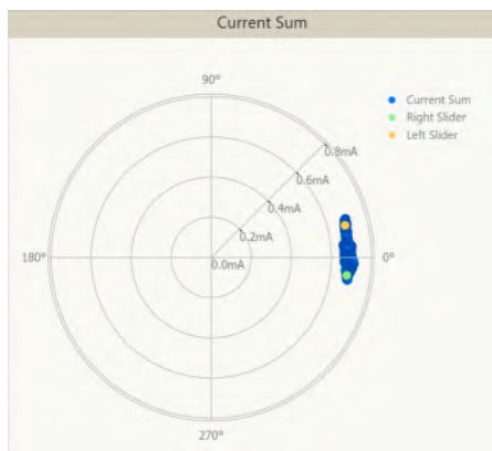
Figure 2. Sum Current Chart for a 650 MVA transformer
