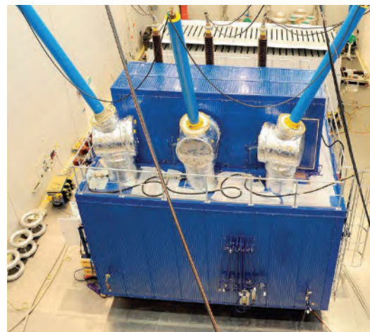
Figure 12. 400 kV transformers with MIDELE 7131 synthetic ester for Highbury substation in London, U.K. (Photo courtesy of Siemens Transformers)
