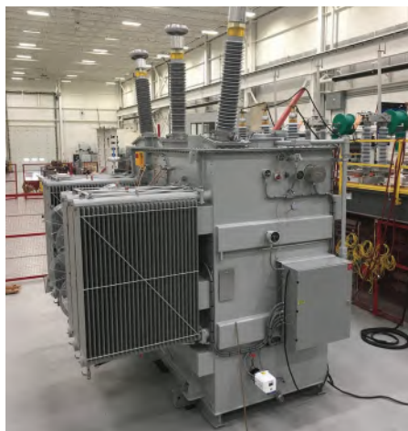
Figure 11. 28 MVA, 138 kV transformer filled with MIDELE n1204 for a mine in Canada. (Photo courtesy of Northern Transformer)
