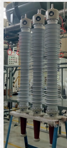
170kV 800A 300BCT
