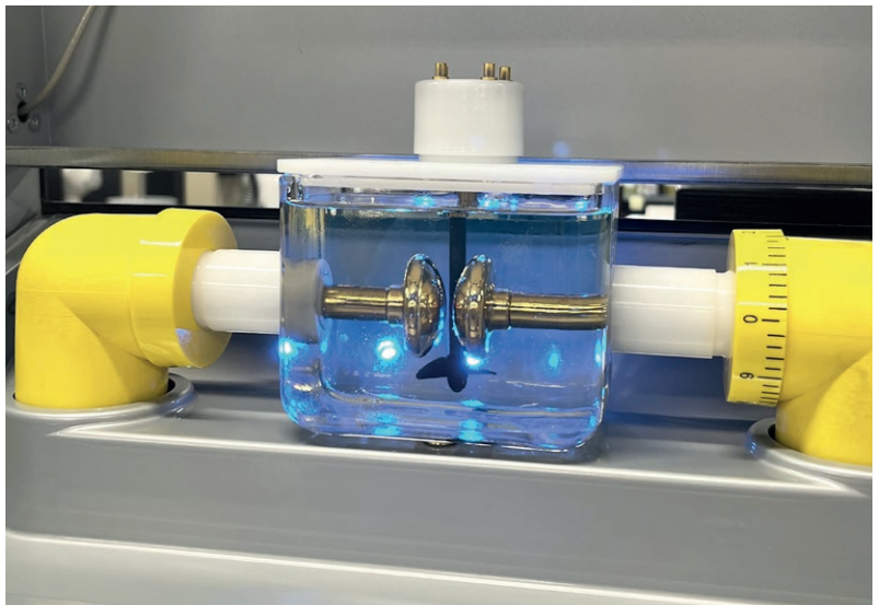
Figure 3: Dielectric Breakdown ASTM D1816
