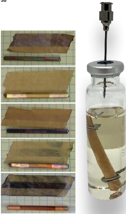
Figure 10: Covered Copper Deposition Testing
