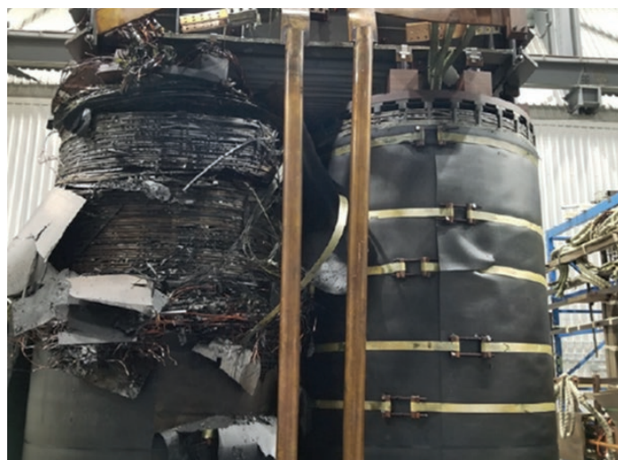
Figure 2. A Single Phase GSU with excessive moisture in the paper, and puncture from HV to LV through the barrier [4]
