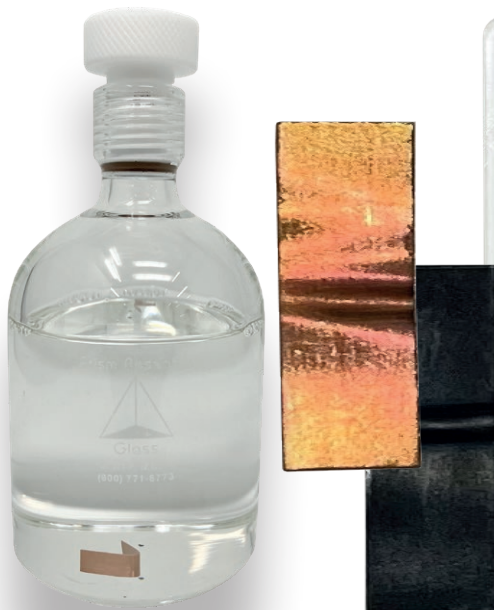
Figure 9: ASTM D1275 Corrosive Sulfur Testing
