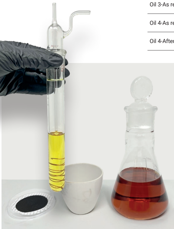
Figure 2: Accelerated Aging Testing ASTM D2440
