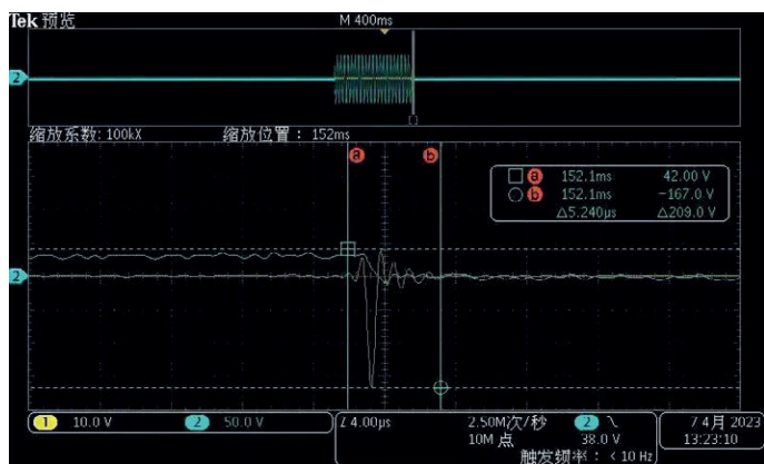
Figure 10: Waveform of Head and Tail Oscillation During Contact Separation -2
