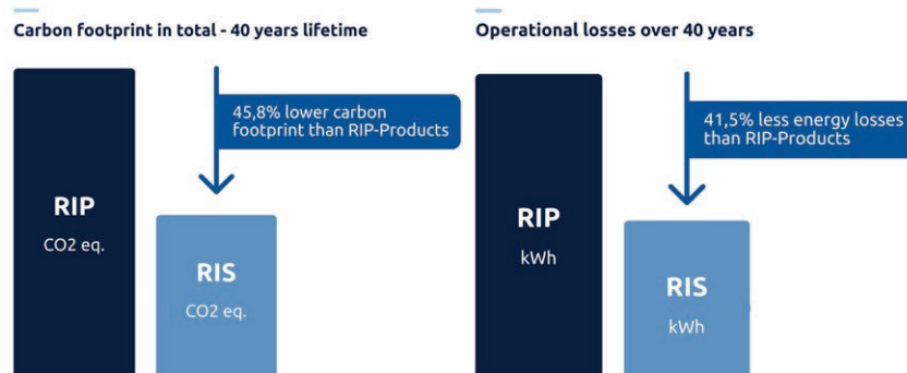
Figure 6: Carbon footprint and operational losses of RIP and RIS condenser bushings
