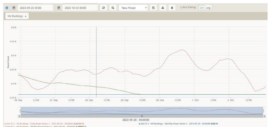
Figure 6: Smoothed Power factor values for a single bushing
