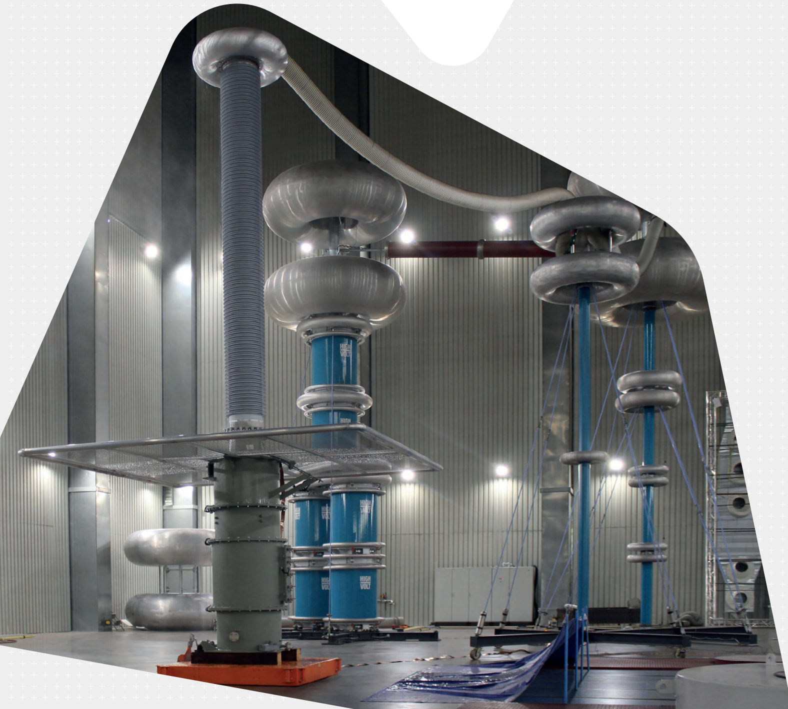
Figure 5: Type test of the 500kV RIS HVDC bushing – Even wetting DC voltage test
