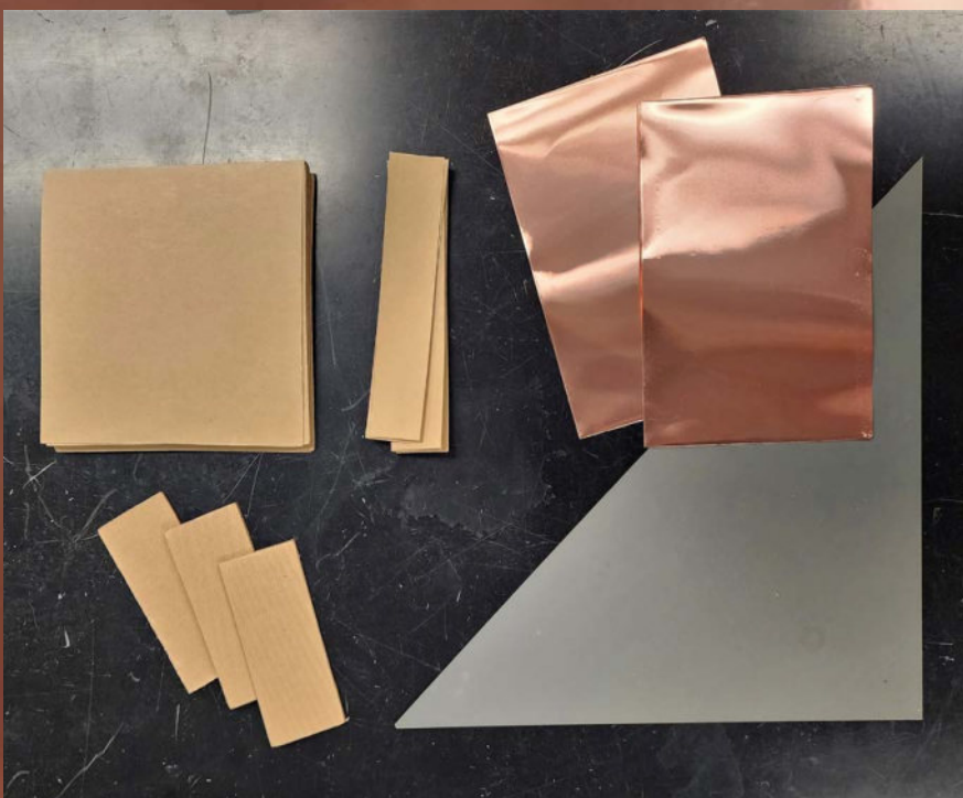
Figure 2: Materials loaded into the aging cell – example
