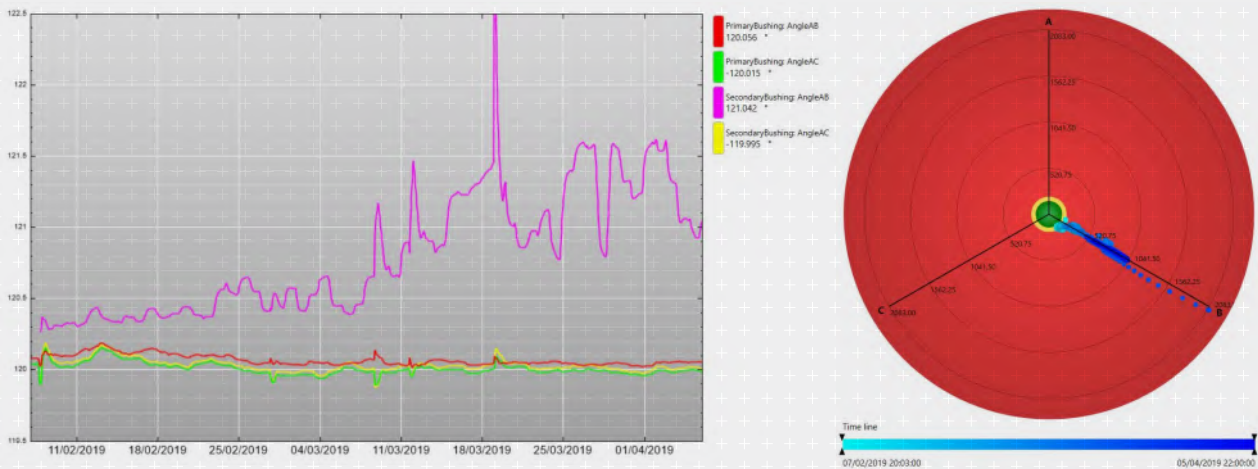
Figure 2. Inter-phase shift increase for LV phase B (indicative of a PF increase): Trend Chart (left); Polar Plot (right)
