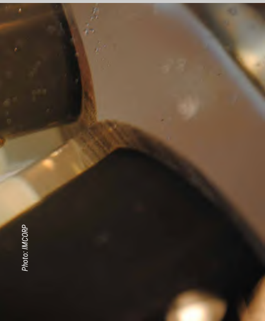
Common manufacturing defect: Protrusion on the inner semiconducting layer of MV cable as seen through transparent insulation during a hot oil analysis
