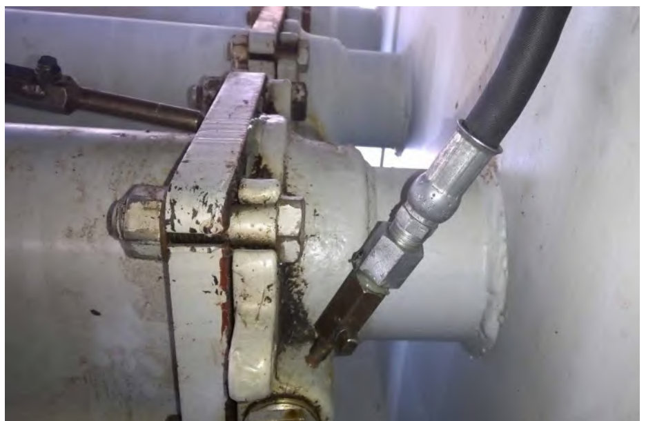
Figure 2. Drill and Inject technique. Left: A graphical sketch depicting how the injection valve is drilled into the gasket groove to inject the liquid sealant material and effectively replace the failed gasket material. Right: Injection valve with sealant injection hose.
