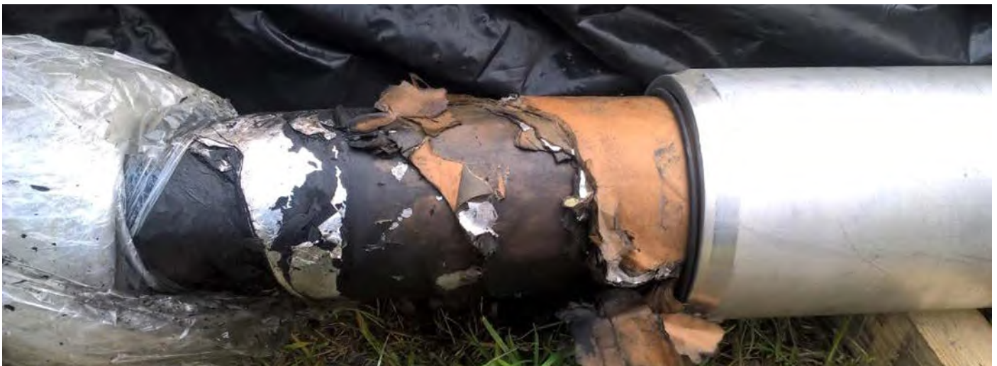
Figure 15. H2 bushing debris found in yard showing failed capacitive layers
