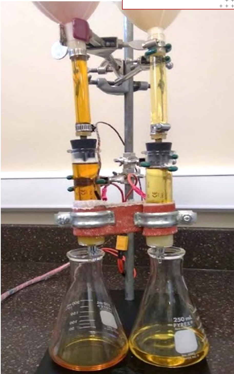
Figure 3. View of the laboratory setup for Fuller's earth reclamation
