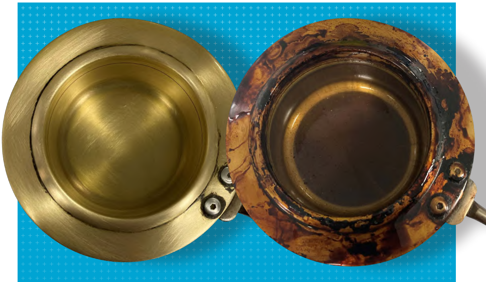
Figure 6. Left: Cup cleaned using wire wool and solvent. Right: No cleaning of cup in between tests
