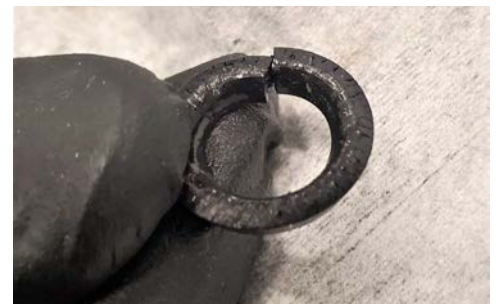
Figure 3. Broken and deteriorated oil fill plug O-ring
