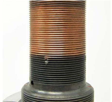
Figure 12. Copper sulfide formation on copper conductor
