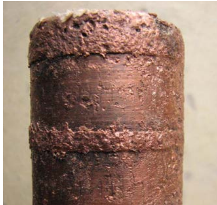
Figure 11. Pitting and melting of copper conductor
