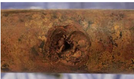
Figure 10. Arc hole through copper conductor
