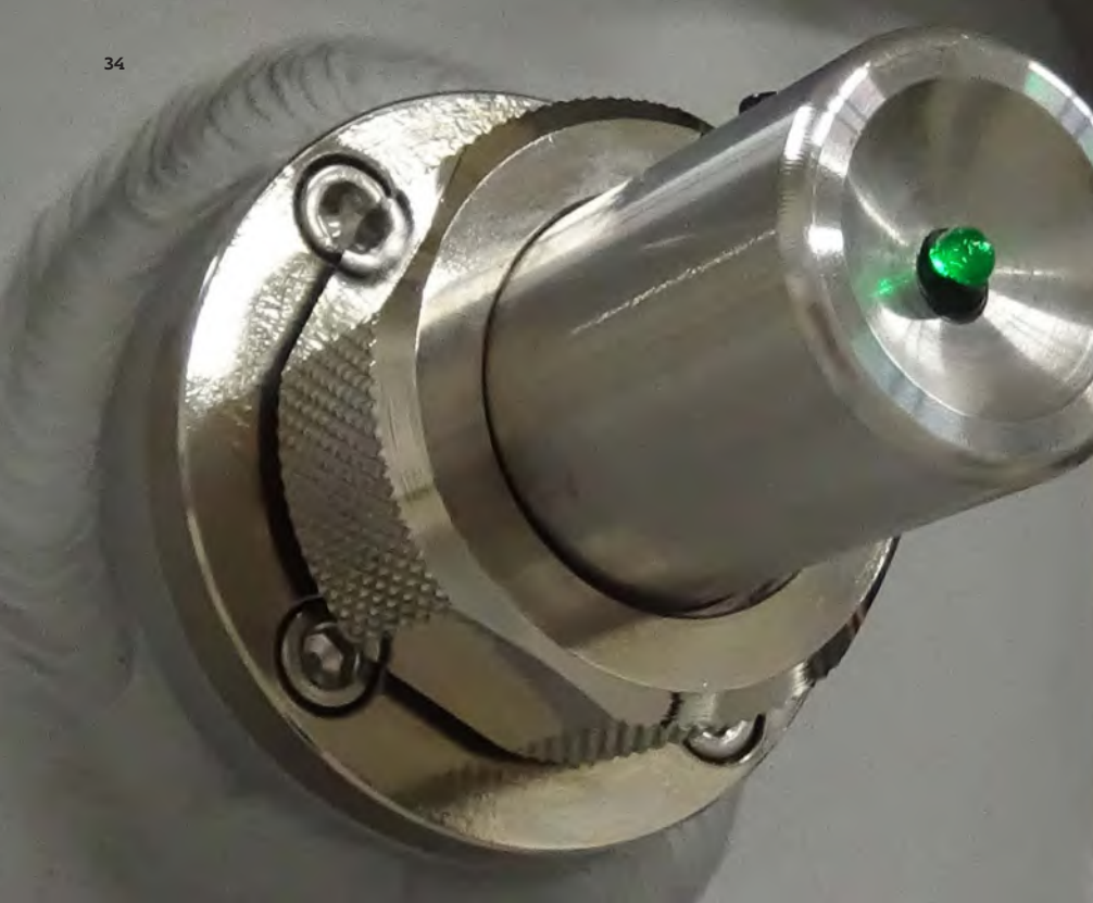
Figure 1. Smart measurement terminal and LED sensor for core insulation condition monitoring
