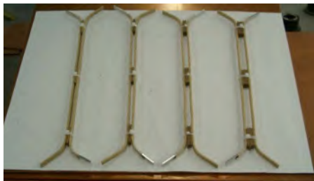
Turn to turn oil gaps, from 3 mm to 12 mm
