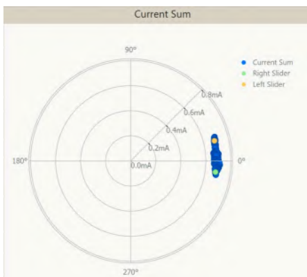
Figure 2. Sum Current Chart for a 650 MVA transformer
