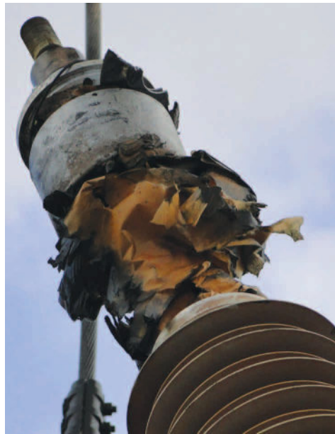
Figure 3. A bushing failure in 2018 had minimal impact on the operation of the substation.
