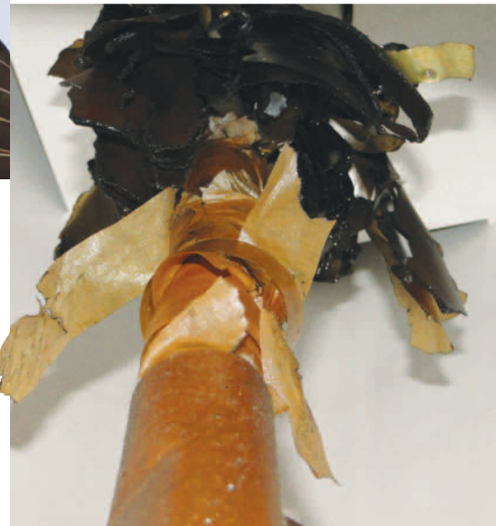
Figure 3. A bushing failure in 2018 had minimal impact on the operation of the substation.
