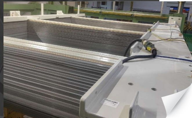
Figure 7. Core loss tests of 50MVA type core at 50 Hz.
