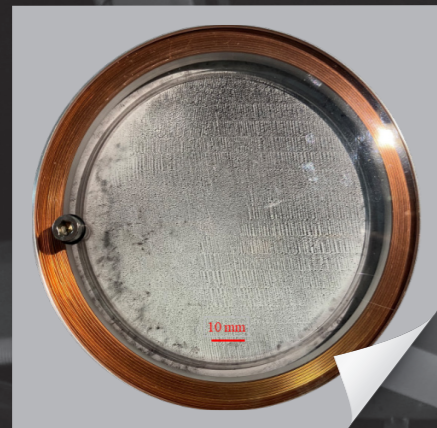
Figure 6. Magnetic domain morphology of 0.18 mm thin-gauge grain-oriented silicon steel.
