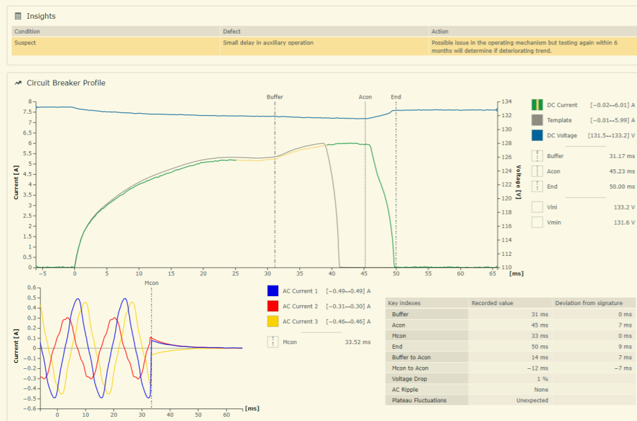
Figure 9: Slower than normal breaker, still good to operate, but with possible issues in the main mechanism
