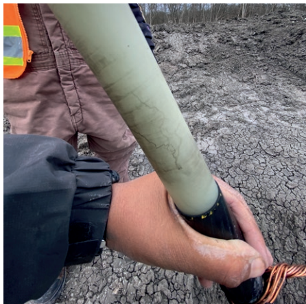
Figure 3 Electrical tree damage resulting from a passing VLF commissioning test.
