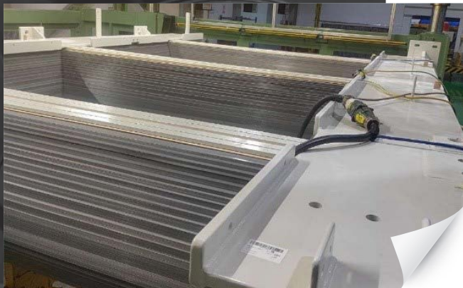
Figure 7. Core loss tests of 50MVA type core at 50 Hz.
