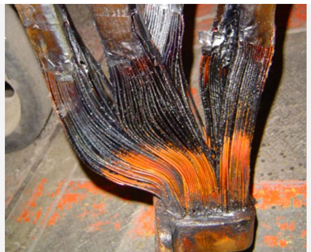
Figure 6: Overheated brazed connections at the bottom end of the LV winding lead.
