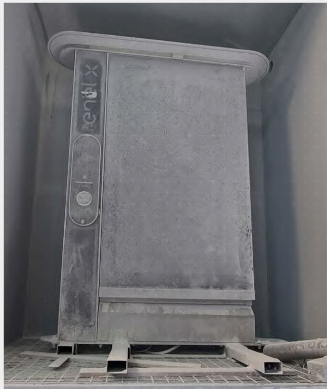
Dust tightness test on charging column
