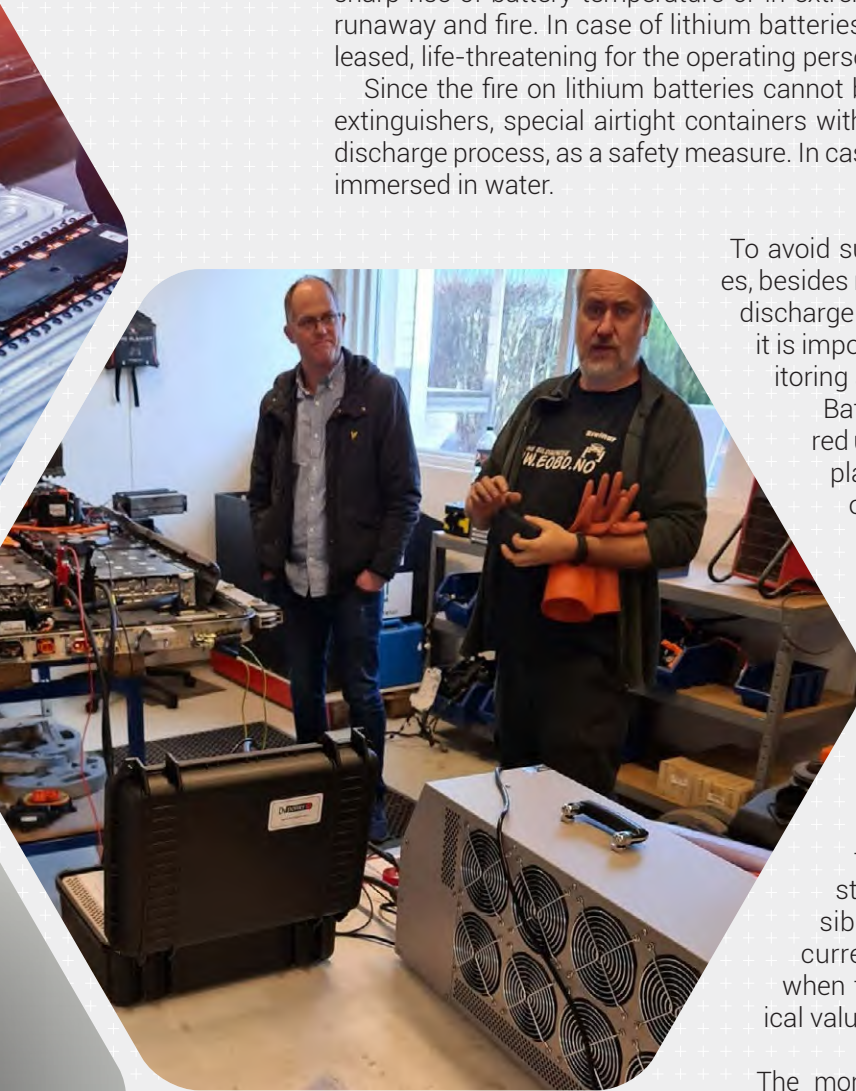
Figure 3. Detached EV battery (left) and Battery load unit BLU360V (right)
