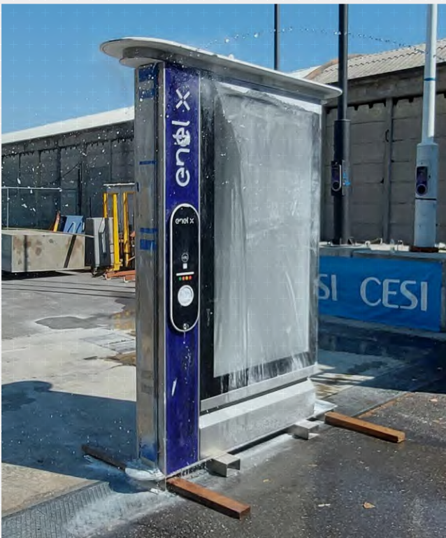
Water tightness test on charging column
