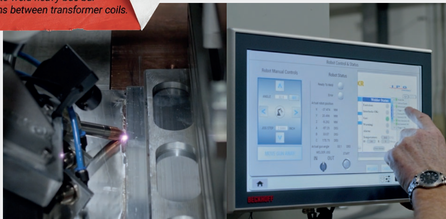
Figure 6: Robotic TIG welding station integrated into a coil production line, used here to weld heavy bus bar connections between transformer coils.
