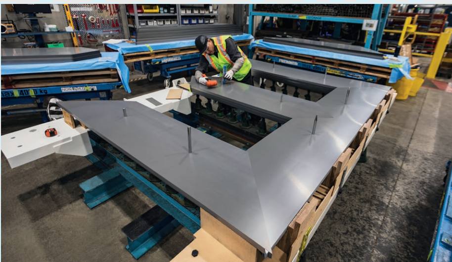
Step Lap Core "E" Assembly
