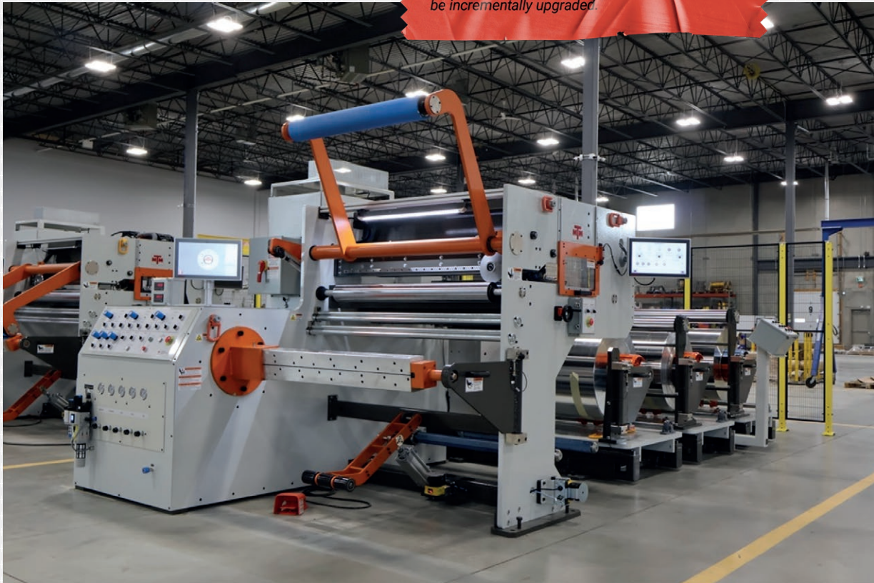
Figure 1: Layout of a combined foil and wire winding machine – a versatile platform that can be incrementally upgraded.
