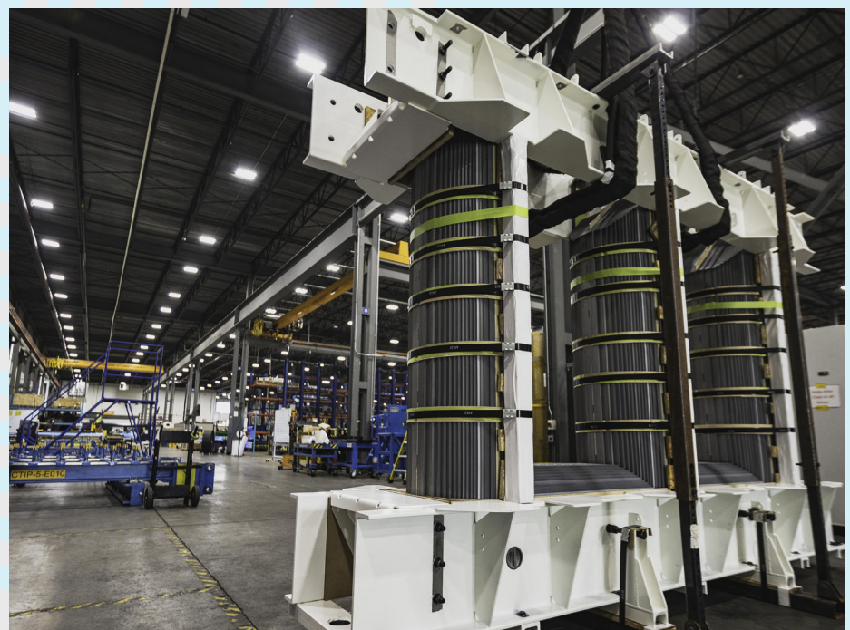
Power Transformer Core
