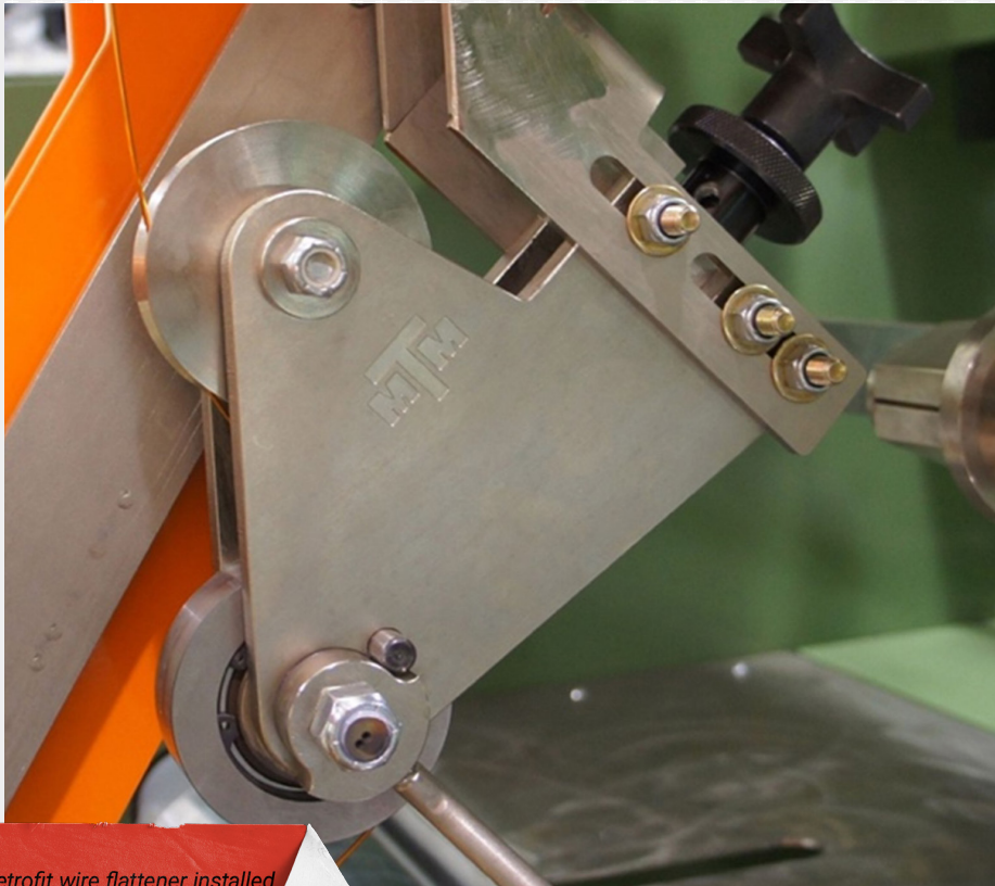
Figure 2: Retrofit wire flattener installed on a coil winding machine to improve winding packing and performance.
