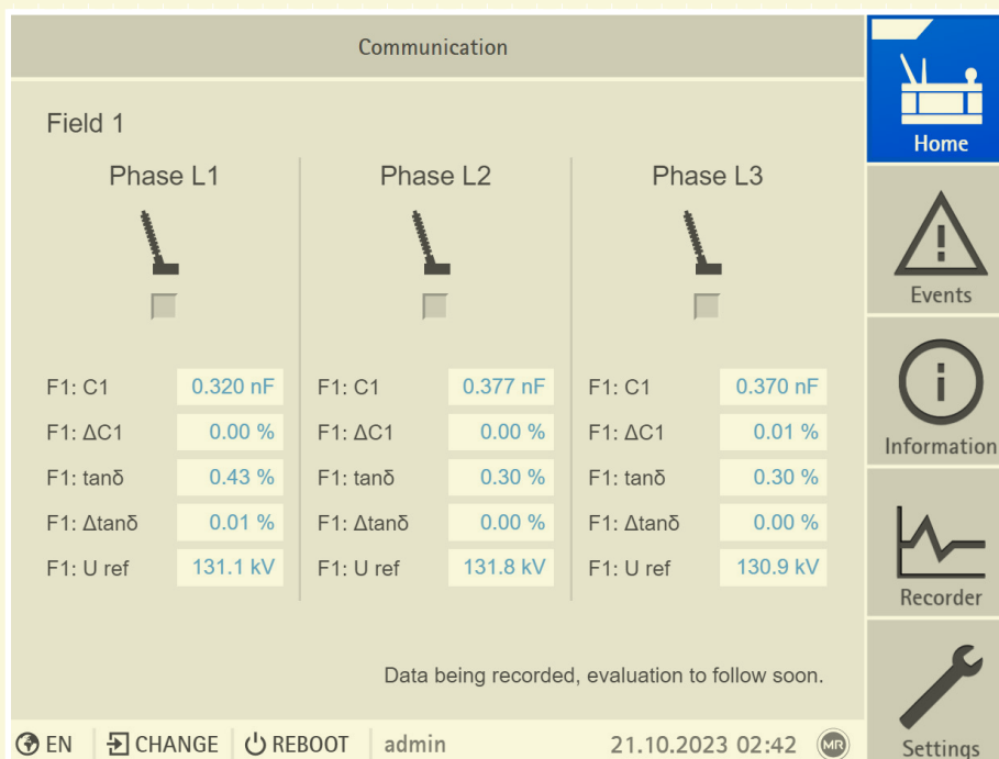
Figure 1: Visualization of the on-line bushing monitoring.
