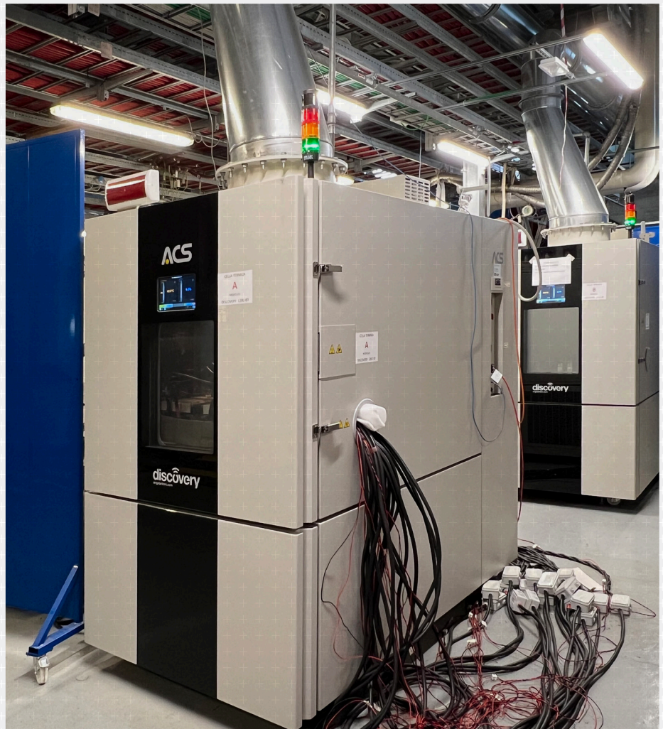
Battery Cyclers for testing EV cells and battery modules
