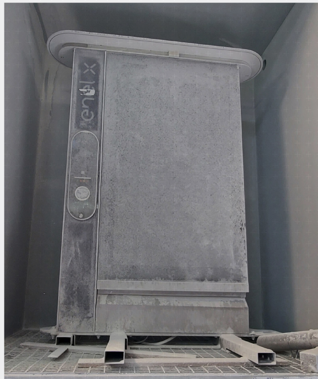
Dust tightness test on charging column
